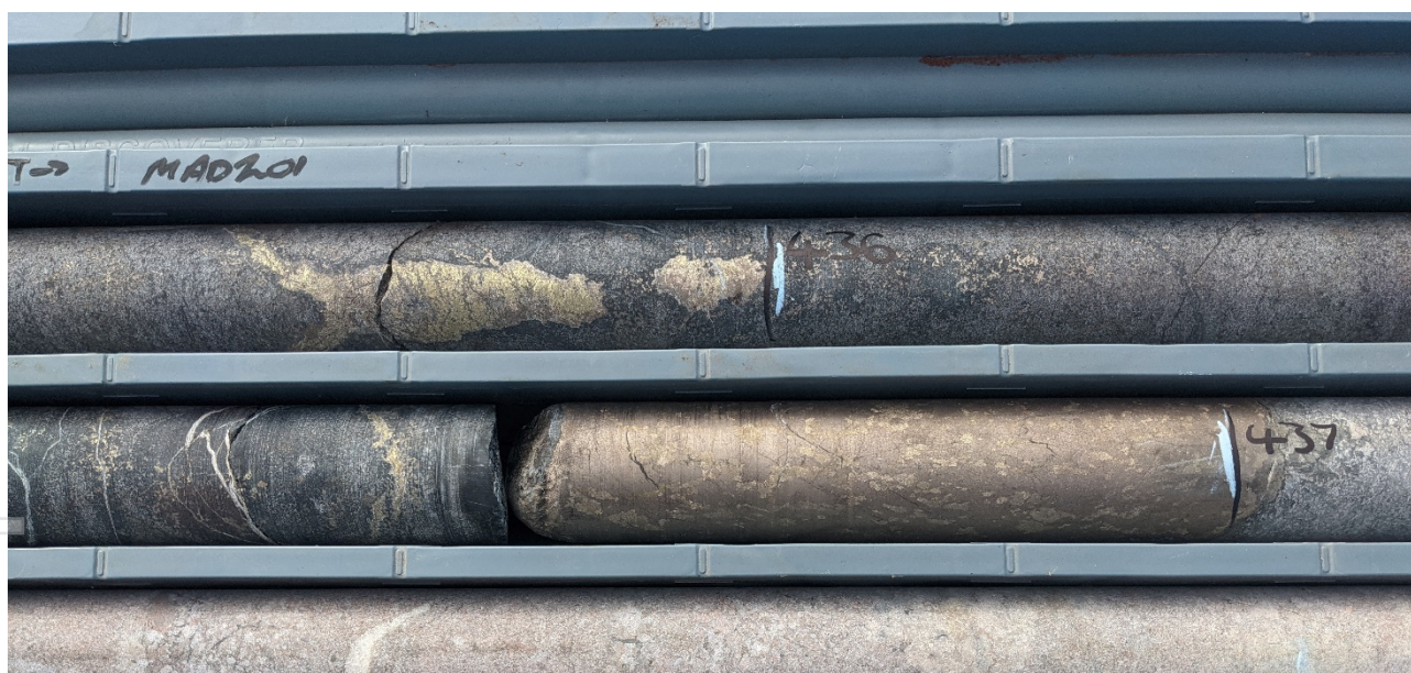
Figure 2 – drill core from the mineralised interval in MAD201 showing massive sulphides as well as stringer and disseminated sulphides. Assays are pending.
